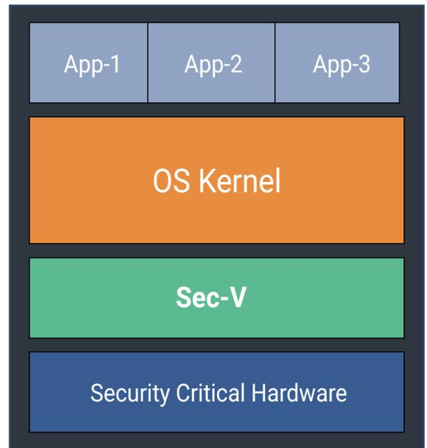
During system boot, Sec-V comes up after BIOS and boots the OS to be protected in a virtual machine. This enables sec-V to set desired security policies on the OS and detect malicious actions performed by malware, even the ones with kernel privileges.
